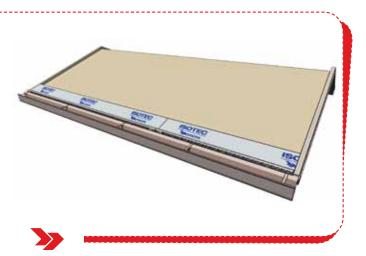
Seal the lateral dovetails of the panels with singlecomponent silicone before their joint. After the panel has been installed and fixed, waterproof the joint with the butyl aluminum tape. Type of fastening are according to the kind of roof structure. Distance is about 1 meter.
