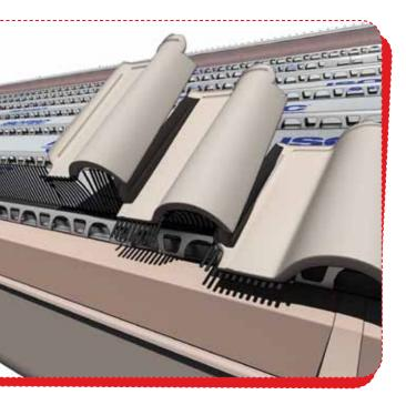
Use the ventilated bird list for eaves along the gutter edge. The height of the bird list ensures the proper inclination of the first row of tiles along the cutter edge (check during tiles laying that combs of the bird list are bent outward). Fixing can be done with other fixing devices, referring to instructions of roof manufacturers or standard rules (i.e. UNI 9460) or local tile laying rules.
