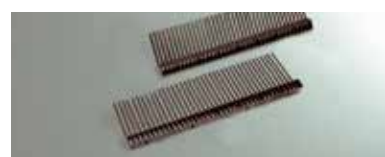
Isotec ventilated gutter batten in polypropylene with teeth 9.5 cm and 12.5 cm, length 38.5 cm
